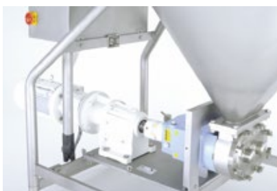
Direct line drive reduces moving parts and increases reliability
