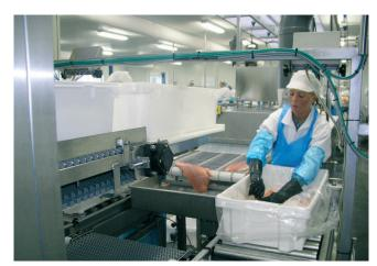
Packing of clean, skinned fillets into boxes after washing and drying.
