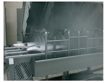
Efficient desliming with Marel Deslimer.
