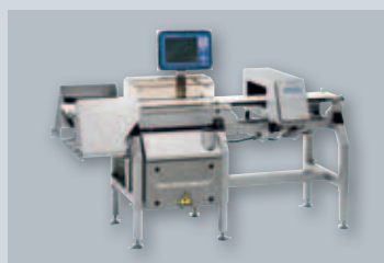
5 The packs pass through a M-Check RF5 checkweigher, which also checks each pack for the presence of any metal. Any packs that deviate from the target weight, or where any metal is detected, are automatically rejected.
