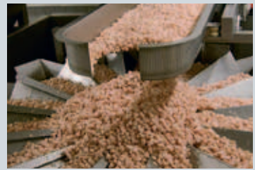
3 The diced ham is dispensed into the hoppers by vibrating feeders and weighed into exact portions.
