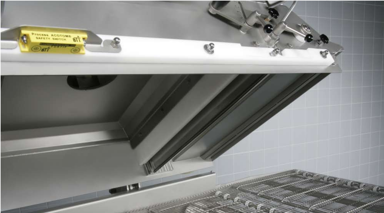
Blower with two adjustable air knives.
