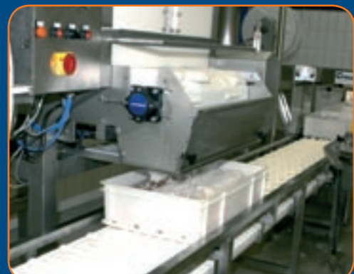
Top icing of boxes with Carnitech Ice Doser type CT 1404.10
