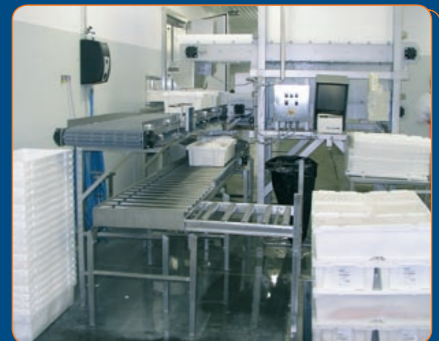
Bottom and top ice with Carnitech Ice Doser type CT 1404.20
