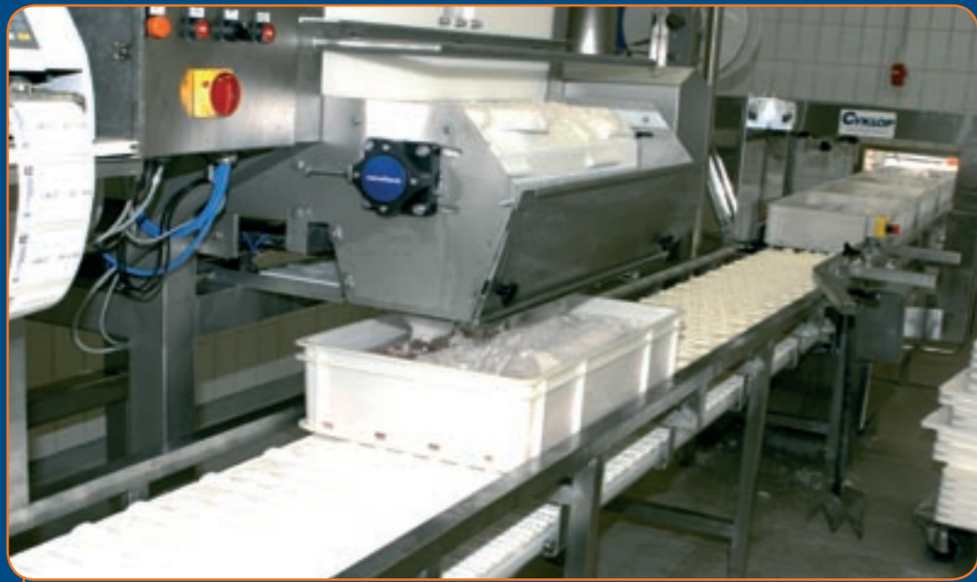
The amount of ice can be adjusted automatically according to different box size
