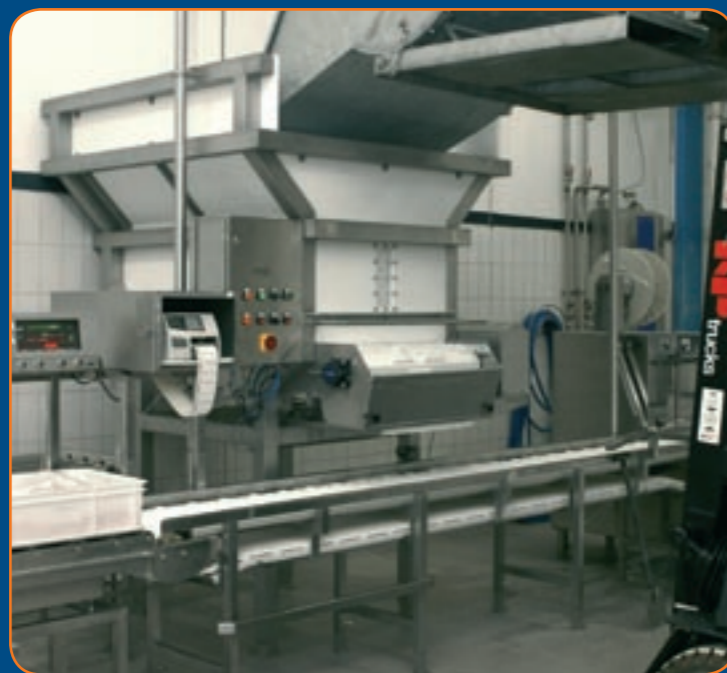
Manual filling of ice into Ice Doser
