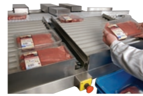
Packing Station Manual crate/box packing & labelling to fixed weight or fixed count. Available in 2 to 16 channels.
