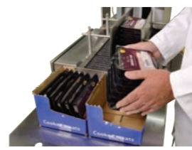
Stacker Indexer Stacks packs to a fixed count to facilitate manual crate/box loading.
