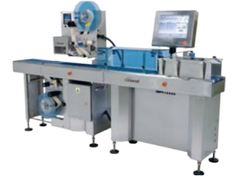
WPL9100 Weigh Price Labeller Versatile, competitively priced, weigh price labeller for speeds up to 100 packs/min.
