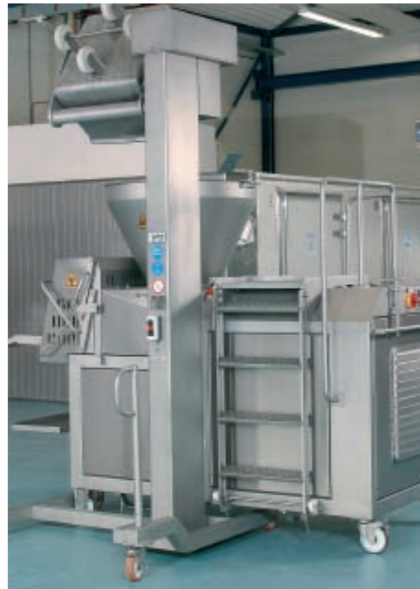
The lifting/tilting unit has been specially designed for the supply and economical loading of the product mass.
