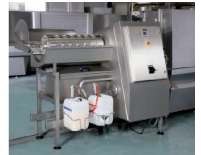
The cleaning unit cleans portioning drums fully automatically both inside and outside.
