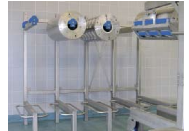
The lifting unit easily moves the portioning drums to the cleaning unit or to the storage rack.
