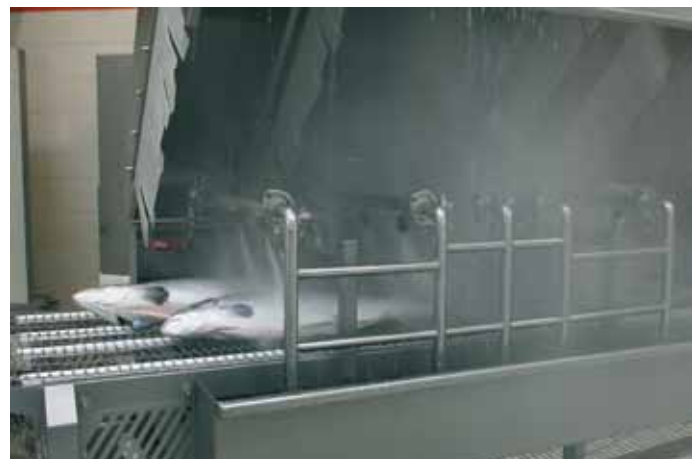
Efficient desliming with Marel Deslimer
