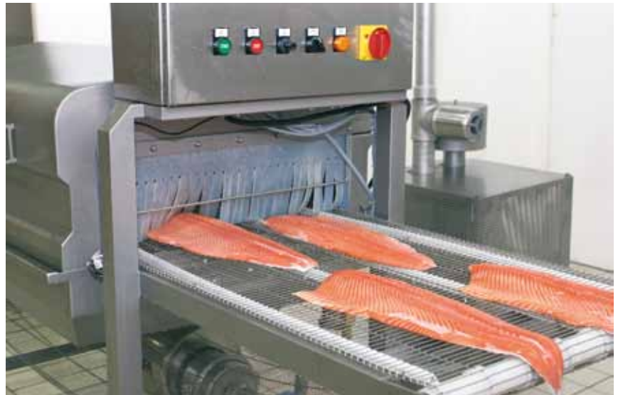
Efficient washing of fillets with Marel fillet washer CT 1636.20
