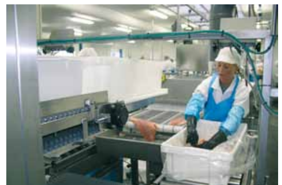
Packing of clean, skinned fillets into boxes after washing and drying
