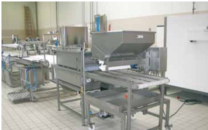
Marel fillet washer integrated into a filleting line
