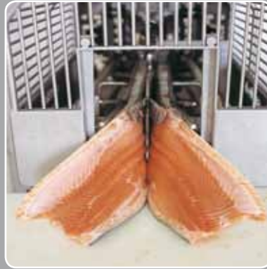
Filleting with the belly bone removed. Fat and white membrane remain on the fillets
