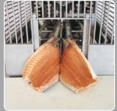
Finished fillet ready for trimming of the edges
