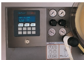
Up to 1000 label comformats can be accessed or edited via the integral keypad.
