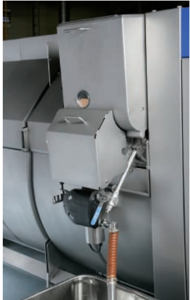
Powder and liquid dosage unit underneath one another fitted to one segment.
