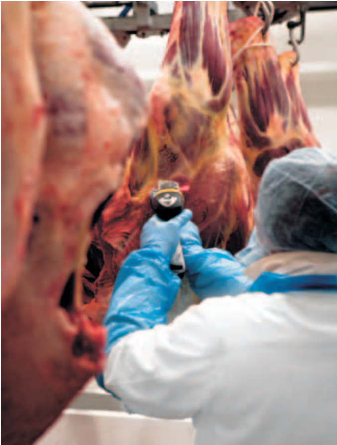
Scanning of carcass information such as type, place of birth and grade
