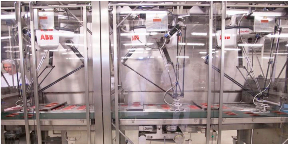
IPL Robot's 3 heads quickly, gently and precisely place sliced groups into the thermoformer at, typically, 180 picks/min.
