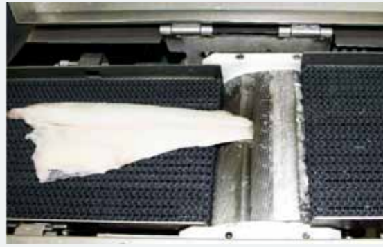
3.2 - Skinning machine: Skinning with minimum yield loss and tear.
