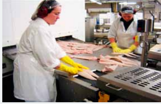
3.1 - Slide to the skinning machine: The product comes from the Super Chiller on a slide to the skinning machine.
