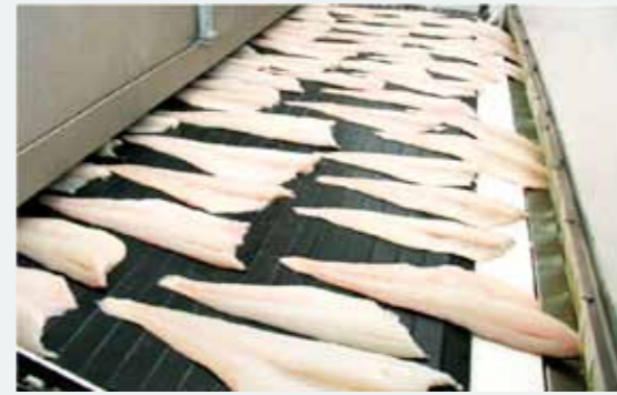
2.3 - Teflon-coated aluminium-droplets belt: The aluminium contact-belt has a flat surface.
