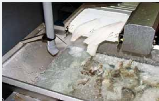
1.2 - Cooling and buffering: The cooling tank acts as a buffer in the processing line.
