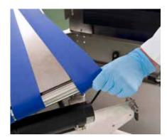
Quick release belts easily removed for cleaning
