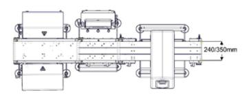
Standard weigh table with metal detector infeed and twin reject shown
