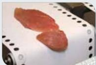
The ultra-fast, rapid-response retraction conveyor opens and closes so quickly that it can even remove trim from both front and back ends of a single product.
