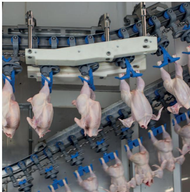
In this context Marel Poultry developed an 8" pitch whole product distribution line, whose distinguishing feature is a shackle which can be turned automatically through 90° and 180° for more accurate weighing and for additional flexibility in where product is unloaded.
