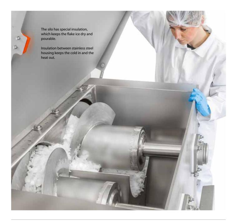
One or several MAJA flake ice machines automatically fill the IXT Silo from the top. Ice machines and silo are integrated to give operators complete control. The ice level indicator and ice production start time can be set via a user-friendly digital display to automatically refill the silo, keep ice levels optimal, and ensure fresh, flake ice is available when needed.
