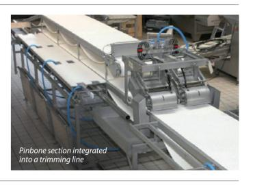
Marel also supplies customized pinbone removers with special features – such as extra length, drip trays, wheels, platforms, etc., designed to meet specific customer needs.
